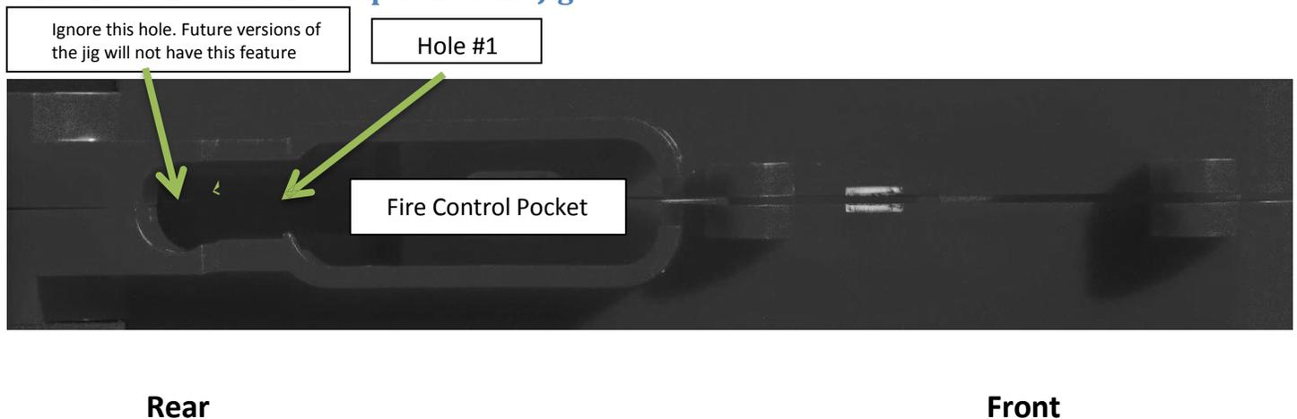
Side View of the Jig, with the Safety, trigger and hammer drill bit holes
