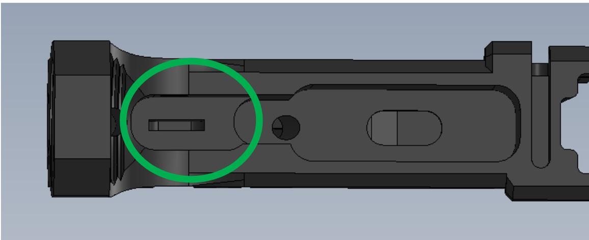
This area near the rear of the Fire Control Pocket is higher or stepped up compared to the deeper pocket. If you have a finished lower receiver from a previous gun, it might be helpful to take compare. You don't need to mill the stepped up area at all, it's done.
