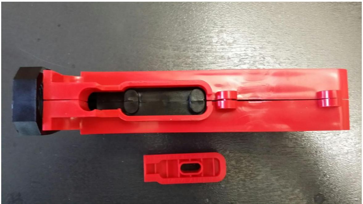
Top view with the Trigger Jig insert which snaps into the top of the jig
